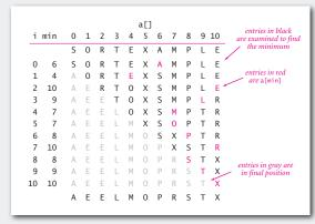
Running time insensitive to input. Quadratic time, even if array is presorted. Data movement is minimal. Linear number of exchanges.
