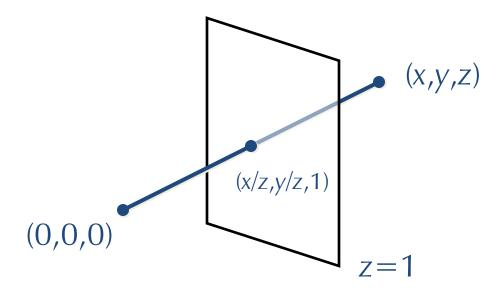
• Add scaling, flipping, etc.  $\Rightarrow$  pinhole camera model
