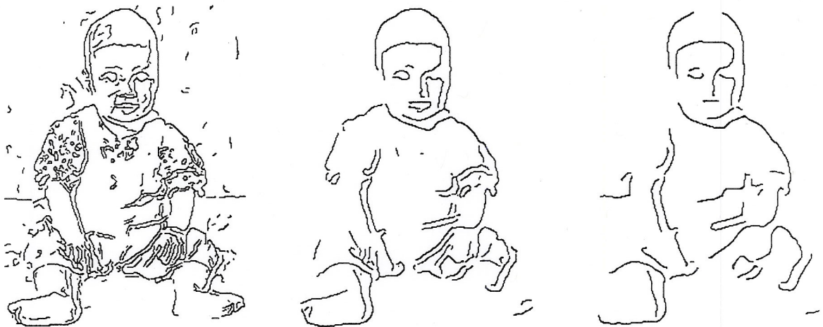
Figure 4.6 Output of HYSTERESIS_THRESH run on Figure 4.5, showing the effect of varying the filter's size. Left to right: \sigma_f = 1, 2, 3 pixel. The grey levels has been inverted (black on white) for clarity.
