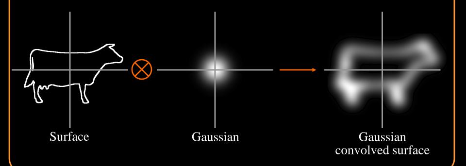
The value at a point is obtained by summing the Gaussian of the closest point on the model surface.
