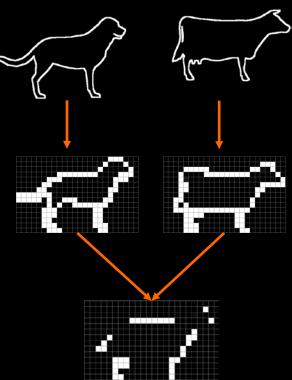
Match by computing the minimal amount of work needed to transform one distribution into the other.
