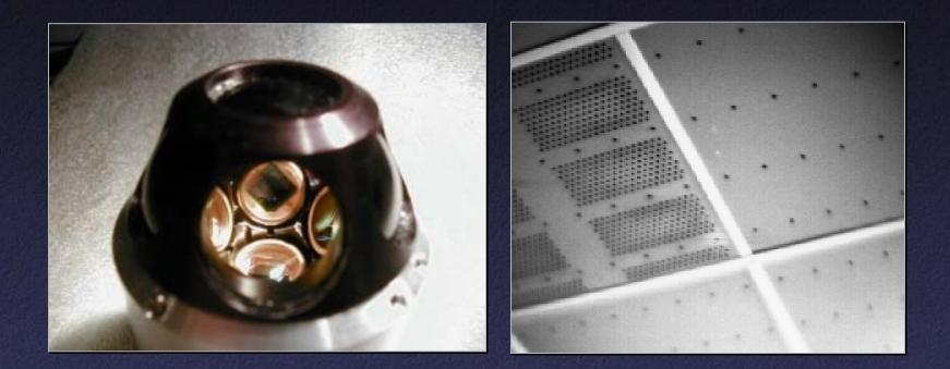
6 cameras, looking at LEDs on ceilingLEDs flash over time
