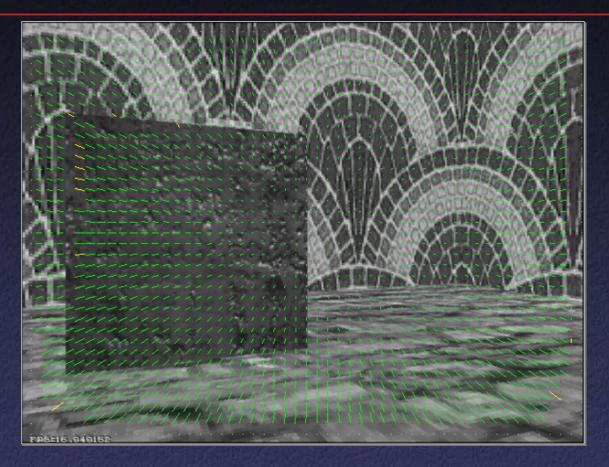
Obstacle Detection: Unbalanced Optical Flow
