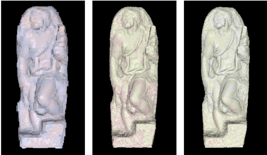
**Figure 6.2:** Streaming within a frame is performed in a series of top-to-bottom sweeps that each download all nodes larger than a certain screen-space tolerance. Here, we show the appearance of the model at three points during refinement. Because the refinement order is based on screen-space size, the splats present within a frame tend to be close to each other in size (as long as the viewpoint is not changed).
