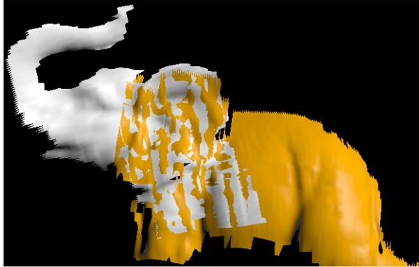
**Figure 3.17:** High-speed ICP algorithm applied to scanned data. Two scans of an elephant figurine from a prototype video-rate structured-light range scanner were aligned by the optimized high-speed algorithm in 30 ms. Note the interpenetration of scans, suggesting that a good alignment has been reached.
