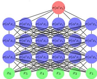
Figure 6.1: A fully connected neural network with 3 hidden layer and an output neuron.
