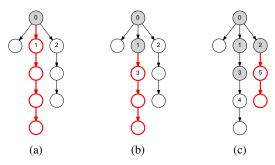
Figure 5: An example of dynamic critical paths during the load of a simple page. Dynamic critical paths are shown in red. Numbers represent the order in which Polaris requests the objects. Shaded objects have been received and evaluated; numbered but unshaded objects have been requested, but have no responses yet. We assume that all objects are from the same origin, and that only two outstanding requests per origin are allowed.
