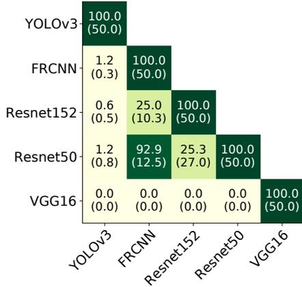
**Figure 2. Percentage of layers that are common among pairs of models, along with the potential memory savings by sharing the common layers in parentheses, e.g., two YOLOv3 models (first row, first column) have all layers in common (hence 100%), and can save 50% memory by merging compared to running individually.**
