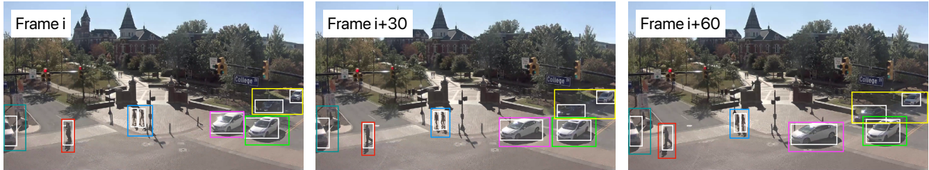
Figure 4: Example screenshots from the Auburn video (Table 1). CNN (YOLOv3+COCO) detections are shown in white, while each of Boggart’s trajectories (and their constituent blobs) is shown in a different color.
