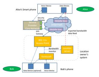
Fig. 1. Architecture of a single-carrier location authentication system.
