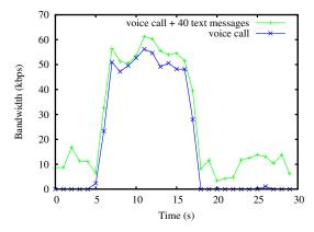
Fig. 2. Average bandwidth measurements captured from our prototype for a 30 second epoch containing an 11 second voice call (blue), and the same call with 40 randomly time-offset text messages (green).
