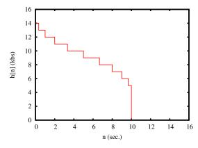
Fig. 5. An example of the bandwidth consumed by a single instance of interfering cross traffic. The duration of a noise burst is 10 seconds.
