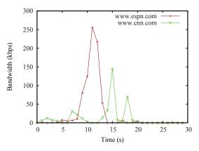
Fig. 4. Average bandwidth measurements for two web page downloads. While some downloads consume high bandwidth and are of short duration (ESPN), others may span a large fraction of the observation interval (CNN).
