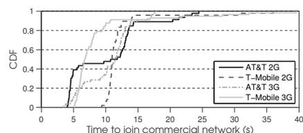
Fig. 9: Time spent without service when moving to commercial networks from a local cell.
