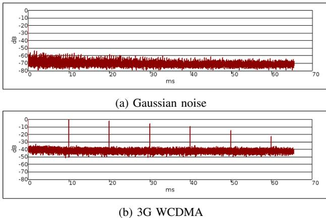
Fig. 2: Peaks with fixed periodicity are observed in the cyclic autocorrelation function, corresponding to timeslots used by cellular synchronization channels.
