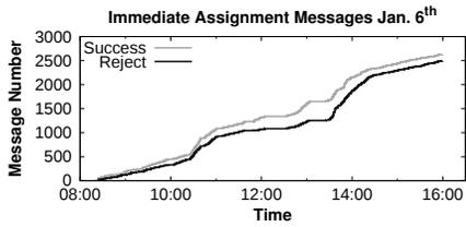
Fig. 4: Successful and failed channel assignment messages collected from Carrier A with different  $\alpha$  values. A over 1 day in Za’atari.
