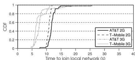
Fig. 8: Time spent without service when moving to the local network from commercial networks.
