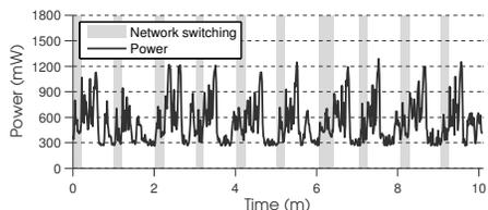
Fig. 7: Energy consumption increases during transitions, but peaks immediately following movement between cellular networks.
