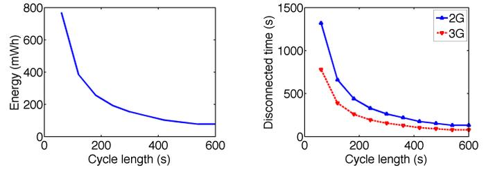
Fig. 3: Power consumption and disconnected time increase exponentially as  $P$  drops close to 15 seconds. As  $P$  increases the energy burden of CellSwitch and the time a phone spends disconnected from both networks decreases.
