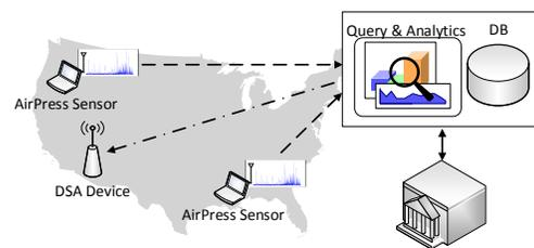
Figure 1: AirPress Overview. Geographically diverse sensors upload spectrum measurements to the spectrum inventory database. A query and analytics engine characterizes these traces. DSA devices and policymakers query the spectrum inventory in order to understand spectrum occupancy.
