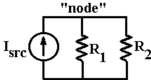
$$I_{src} - I_{R1} - I_{R2} = 0 \text{ (sum of currents must } = 0) \quad I_{src} - V/R_1 -$$
