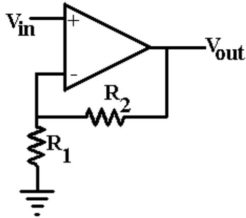
$$i_{R_1} = i_{R_2} = \frac{v_-}{R_1} = \frac{v_+}{R_1} = \frac{v_{in}}{R_1}$$
