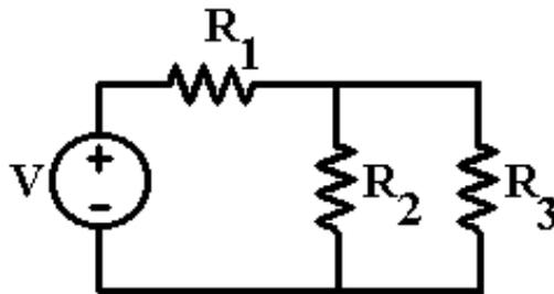
What's  $V_{R_2} = V_{R_3}$  ?
