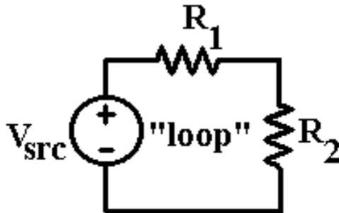
$$V_{src} - IR_1 - IR_2 = 0 \quad (\text{currents must all be same})$$
