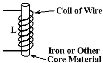
Current in coil causes magnetic field, which stores energy.
