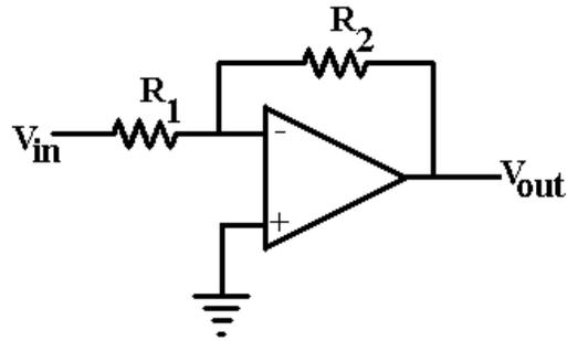
$$v_{out} = i_{R_2} R_2$$
