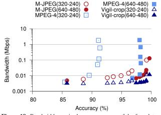
**Figure 18:** Bandwidth required versus accuracy of the face detection vision algorithm on videos compressed with different video compression algorithms, including our algorithm Vigil-crop that performs M-JPEG on the cropped objects. Only the selected frames in the sis array are compressed for this bandwidth calculation.
