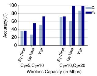
**Figure 17:** Accuracy of a multi-cluster system with 10 clusters where the wireless capacity of 5 clusters is  $C_1$  and other 5 clusters  $C_2$ . Vigil outperforms both equal time-based fairness (Eq-Time) and equal throughput allocation (Eq-Thrpt).
