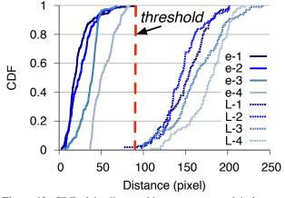
**Figure 19:** CDF of the distance l between two people's faces and the projection errors e when mapped from one camera view to another (illustrated in Figure 7(b)).
