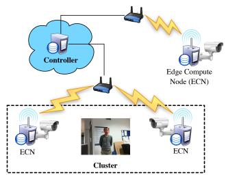
**Figure 3:** Vigil architecture, in which *Edge computing nodes* (*ECN*) are connected to camera devices to perform simple vision analytic functions, while uploading a relevant portion of video feed to a *Controller* in the Internet. Cameras monitoring the same areas form a *cluster*.
