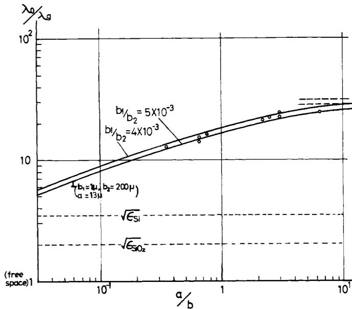
Fig. 4. Slowing factor versus width-to-height ratio  $a/b$ . Open circles: experimental values. Solid lines: theoretical values. Dashed lines: slowing factor in the infinitely wide strip case. 1: delay data in [2].
