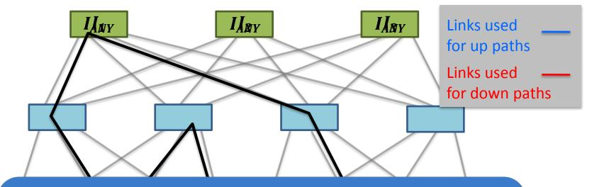
[ IP anycast + flow-based ECMP ]
