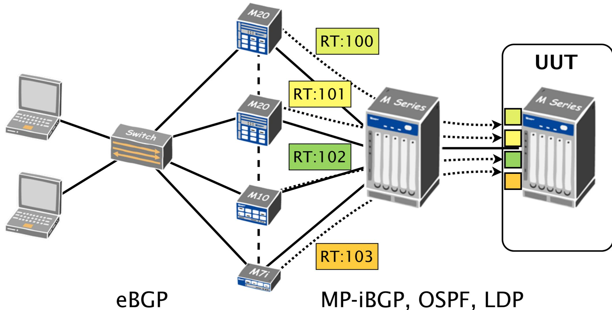
Four services are defined on the Unit Under Test (UUT)
