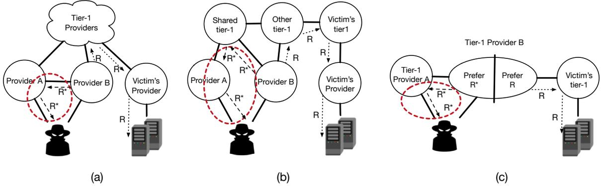
**Figure 3:**  $R^*$  (dashed lines) and  $R$  (dotted lines) learned by  $B$  in three different cases: (a) The adversary has two non-tier-1 providers that peer with each other. (b) The adversary has two non-tier-1 providers that share a common tier-1 provider. (c) The adversary has two tier-1 providers. The red cycles highlight the route  $B$  prefers.
