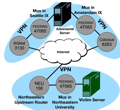
**Figure 7: Experimental setup to launch BGP attacks at Seattle and forward traffic through Coloclue.**
