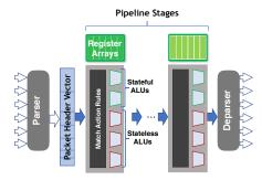
Figure 2: Protocol Independent Switch Architecture (PISA)
