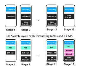
(b) Switch layout with forwarding tables, ACL tables, CMS, and Bloom filter used in stateful firewall.
