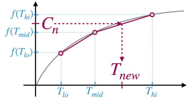
Fig. 5. Finding new bandwidth limit using interpolation. When we plot  $f(T_*)$ , x-axis in this figure refers to the bandwidth limit  $T_*$  (y-axis in Fig. 4), while y-axis in this figure refers to the area under line  $T_*$  in Fig. 4.
