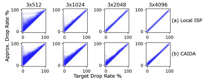
Fig. 12.  $3 \times 4096$  CMS-LPF estimator is sufficient for serving millions of users, with negligible error in drop probability.
