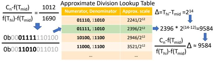
Fig. 6. We use a lookup table to implement approximate linear interpolation. We first match on the highest binary bits of numerator and denominator to get a scaled division result, then multiply  $\Delta$  via bit shifting for the final result.
