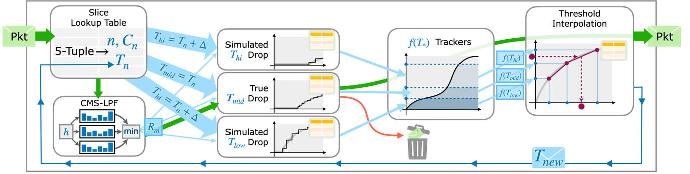
Fig. 3. When a packet arrives, AHAB first maps it to a slice  $n$  and estimates its user's sending rate  $R_m$  using the CMS-LPF estimator (§IV-B), then uses probabilistic dropping to enforce slice  $n$ 's bandwidth limit  $T_n$  (§V-A). AHAB also maintains two bandwidth limit candidates  $T_{low}$ ,  $T_{hi}$  and tracks the hypothetical total bandwidth usage  $f(\cdot)$  (§V-B), which is used to derive a more accurate bandwidth limit  $T_{new}$  via approximated linear interpolation (§V-C).
