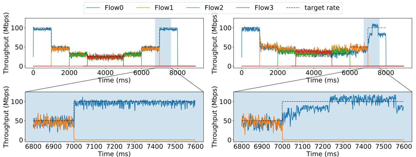
Fig. 7. AHAB (left) converges to fair bandwidth allocation within 3.1ms on average, while HCSFQ [21] (right) needs 42.3ms.
