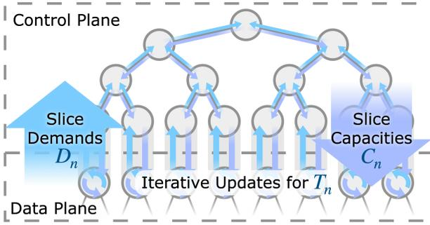
Fig. 2. The control plane maintains inter-slice fairness by periodically reading each slice bandwidth demands  $D_n$  and writing fair capacities  $C_n$ ; the data plane keeps intra-slice fairness by iteratively updating bandwidth limits  $T_n$ .
