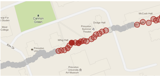
Fig. 11. A student uses a ECCP-enabled phone to stream music while walking across campus. The phone migrates the connection between available WiFi (red) and cellular 4G (gray) networks, without loss of playback quality. The opacity of each data point is an indicator of the throughput (relative to the interface medium) achieved at that location.
