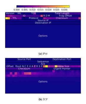
**Figure 5:** Per-bit feature importance for passive OS detection. Brighter colors are more important. Given the nPrint representation, ML models can automatically discover important features (e.g. IP TTL, window size), as opposed to relying on manual engineering.
