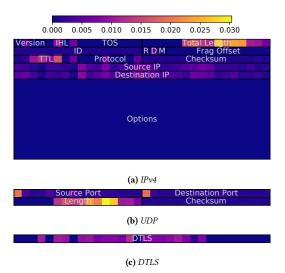
**Figure 8:** Per-bit feature importance for (browser, application) identification, computed by summing the feature importance for each individual nPrint in the 43 packet nPrint created for each handshake. Brighter colors are more important. Given the nPrint representation, ML models can automatically learn important features (e.g., length), as opposed to relying on manual engineering.
