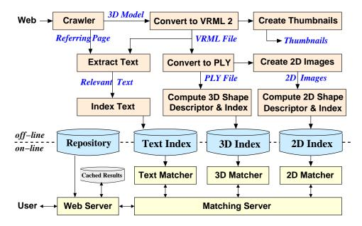
Fig. 11. Flow of data through the search engine. The data shown in blue text is stored in the repository.
