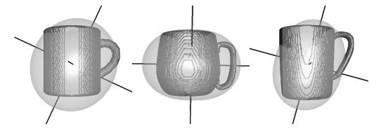
Fig. 3. A collection of mugs drawn with their principal axes. Despite the similarity in the models, the principal axes orient the models in very different ways.
