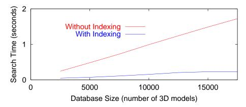
Fig. 14. Search times (in seconds) for spherical harmonics with/without indexing.
