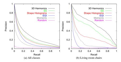
Fig. 13. Plots of precision versus recall of our spherical harmonics descriptor versus other shape matching methods.
