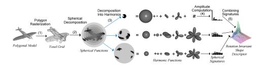
Fig. 4. Computing our spherical harmonics shape descriptor.
