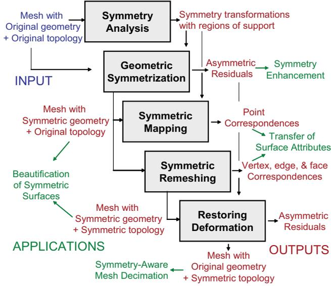
Fig. 1. Symmetry-aware mesh processing framework.
