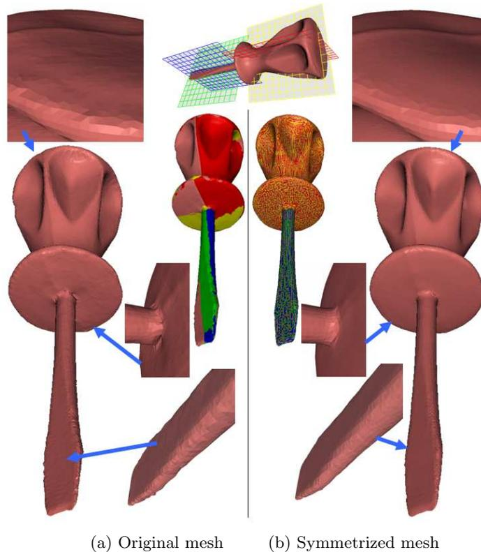
**Fig. 7.** Symmetrizing a scanned screwdriver model. The input mesh is shown on the left side, and the output mesh is on the right. Note that the output mesh is perfectly symmetric, has less noise (e.g., on the tip and at the junction with the handle), and retains sharp features (e.g., the ridge on the top of the handle).
