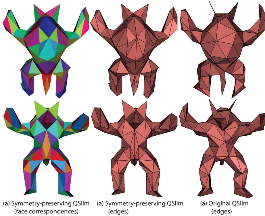
**Fig. 10.** Symmetry-preserving QSlim (a-b) produces a surface approximation comparable to the original algorithm (c) of [19], but guaranteed to have symmetric topology, even for an asymmetric surface (the first column (a) shows symmetric face correspondences preserved during the decimation).
