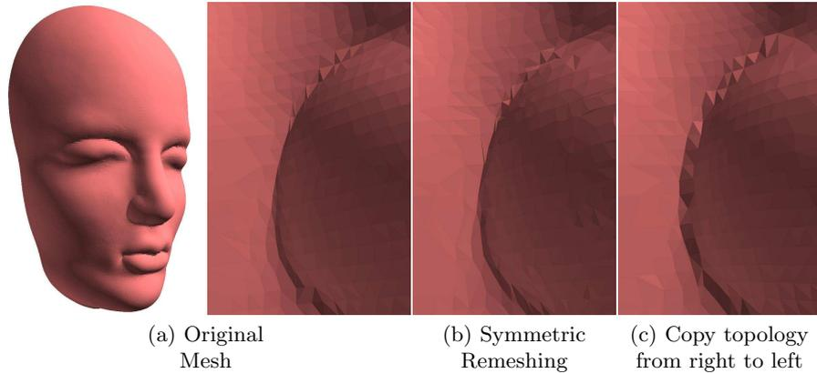
**Fig. 6.** A zoomed-in comparison the crease along left side of the nose on the surface of the mask shown on the left. Note how our approach (b) does not produce blurring when compared to the original (a), while the simple alternative (c) of copying topology from one side to the other does.
