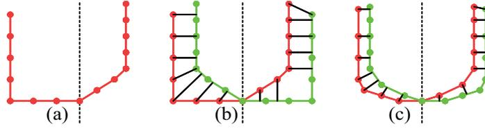
**Fig. 2.** Schematic of one iteration in our symmetrization process (in 2D). (a) Given a curve (red) and a symmetry transformation (reflection across the dotted line), (b) we find correspondences between vertices and the closest point on the reflected curve (green), and (c) solve for new vertex positions that minimize an error function based on those correspondences.
