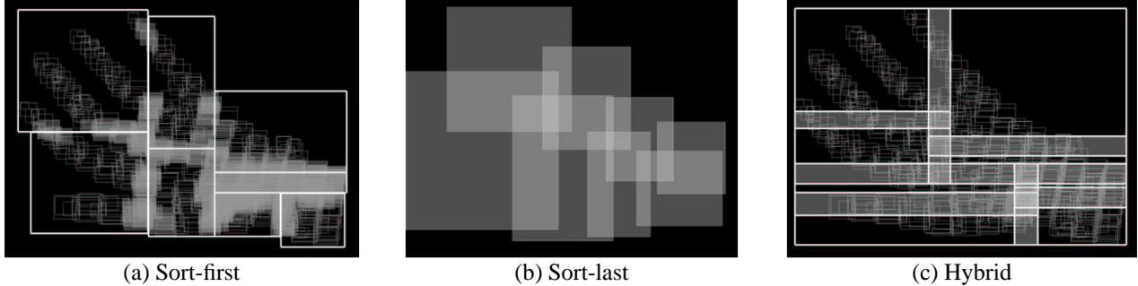
Figure 1: Visualizations of overheads during parallel rendering of hand with different algorithms. In (a), highlighted object bounding boxes span multiple tiles and must be rendered redundantly. In (b) and (c), brighter pixel intensities represent more image composition overheads.
