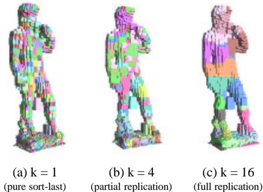
Figure 3:  $K$ -way replication ( $k = 4$ ) enables view dependent partitioning without full replication. Color of each bounding box indicates which server renders its enclosed triangles.
