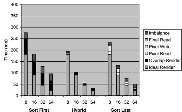
Figure 2: Server time breakdowns for sort-first, sort-last, and the hybrid algorithms for screen resolution 1280x960. The height of each bar represents the time required for processing in the server.
