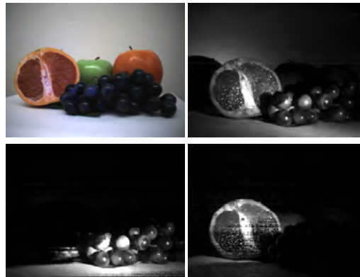
Figure 1. Row 1: Images of a scene captured with regular vision camera under ambient lighting (left) and a single-photon sensitive SPAD array under diffused laser illumination (right). Row 2: The temporal response approximately 703 ps (left) and 1171 ps (right) after emitting a pulse of light into the scene.
