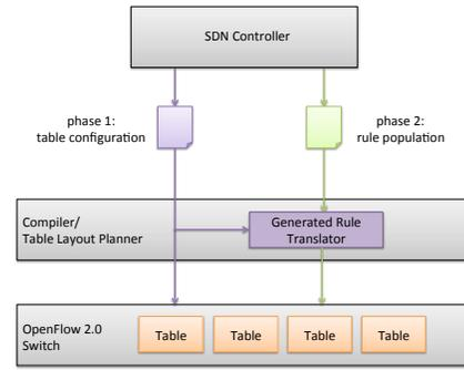
Figure 1. Architecture of an OpenFlow 2.0 System
