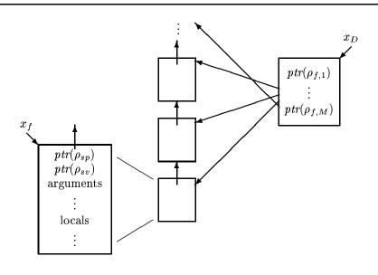
Figure 7: Snapshot of the stack and display during the execution of a translated program.
