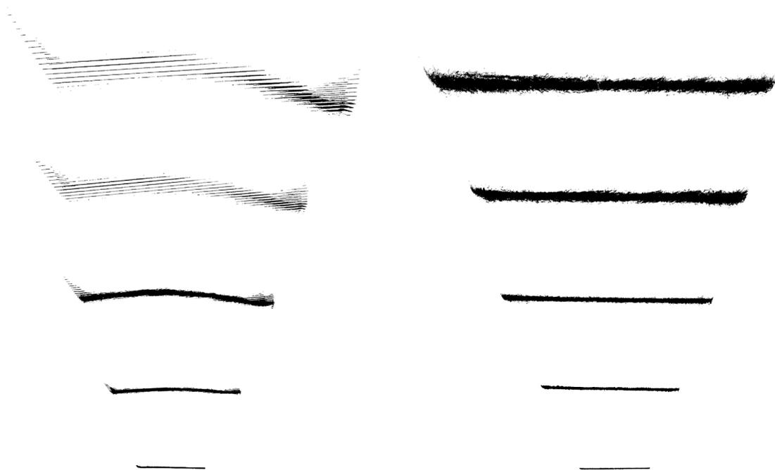
Figure 3.9: Visualization of depth maps of a flat wall, captured at different distances (one to five meter range) **Left:** Raw depth maps. **Right:** Undistorted depth maps.
