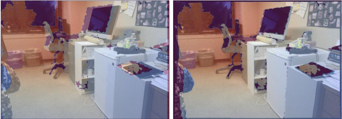
Figure 3.8: Before-and-after comparison of the estimated depth-to-color alignment. In the overlay images, It is easy to see that without calibration the objects in both images do not align correctly.
