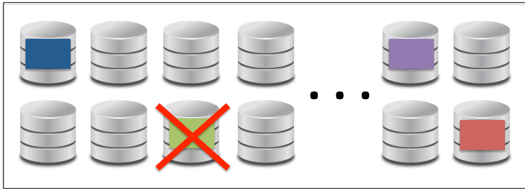
Figure 1.2: Durability is a property that guarantees that hardware failures do not result in data loss. For example, if the indicated machine crashes, the distributed system should still be able to recover the green data block.
