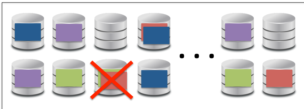
Figure 1.3: Replication ensures that data blocks are still preserved despite some number of failures.
