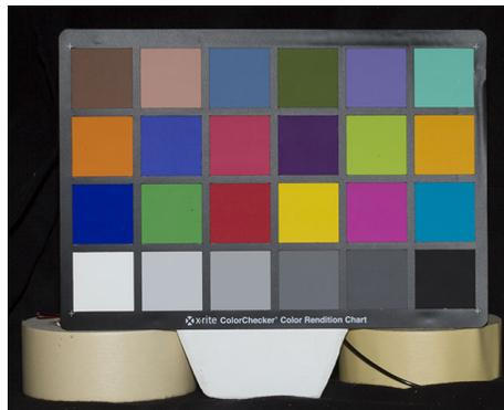
Figure 2.12: **Albedo acquisition of the Penguin:** An X-rite color-checkerboard is used for color calibration and albedo estimation.
