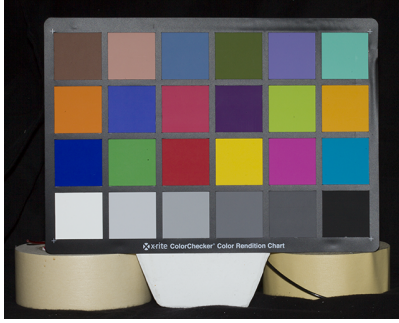
Figure 2. Albedo acquisition of the Penguin: An X-rite color checkerboard is used for color calibration and albedo estimation.
