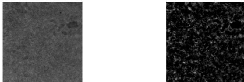
(a) Concrete Patch without Band Pass Filter (b) Concrete Patch with Band Pass Filter
