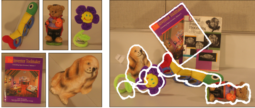
Figure 7.5: Detecting objects. Templates, left, are matched to the image, right. Square patches are matched, searching over all rotations and scales, as described in Section 3.5. A similarity transform is fit to the resulting correspondences using RANSAC.
