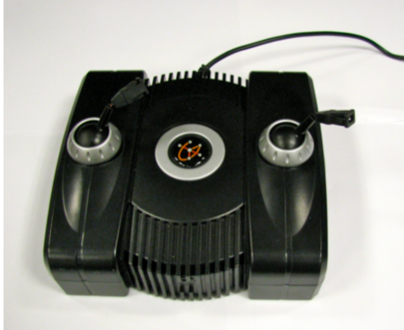
Figure 4.1: The GameTrak Real World Golf USB controller. The base unit houses two spring-loaded strings that can be pulled out from the base and moved in 3D space. The unit can be employed as a 6-axis HID device (x-, y-, and z-axes for each string). The controller also includes a detachable button that can be pressed using the foot.
