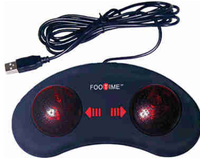
Figure 3.24: The Footime USB controller, produced by Bili Inc., used for hands-free control of Wekinator recording and running.
