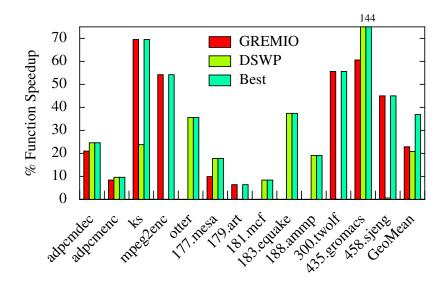
Figure 6.5: Speedups for dual-thread GREMIO and DSWP over single-threaded execution.
