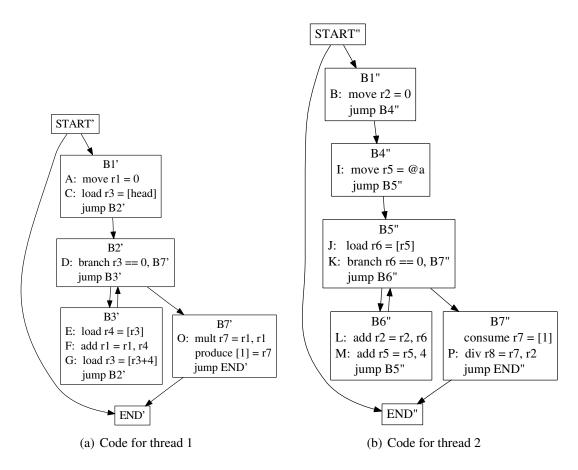
Figure 5.4: Resulting multi-threaded code.
