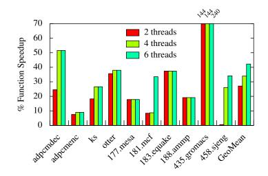
Figure 6.8: Speedups for DSWP over single-threaded execution.
