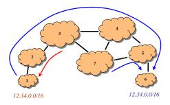
Figure 1: Announcement of prefix 12.34.0.0/16 from two origins partitions the network into two subsets.
