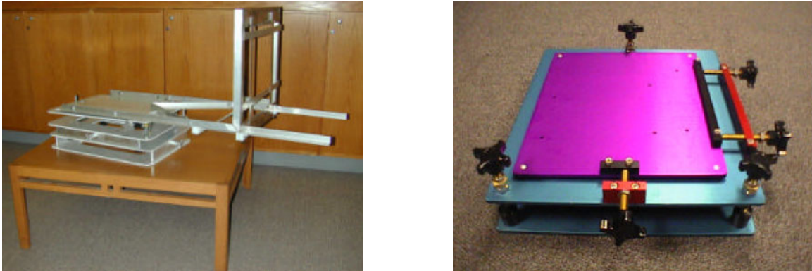
Figure 5.1: Manually Adjustable Projector Mounts with Six Degrees-of-Freedom. Left: mount designed by Princeton University and manufactured by Intel. Right: an improved design by Argonne National Laboratories.
