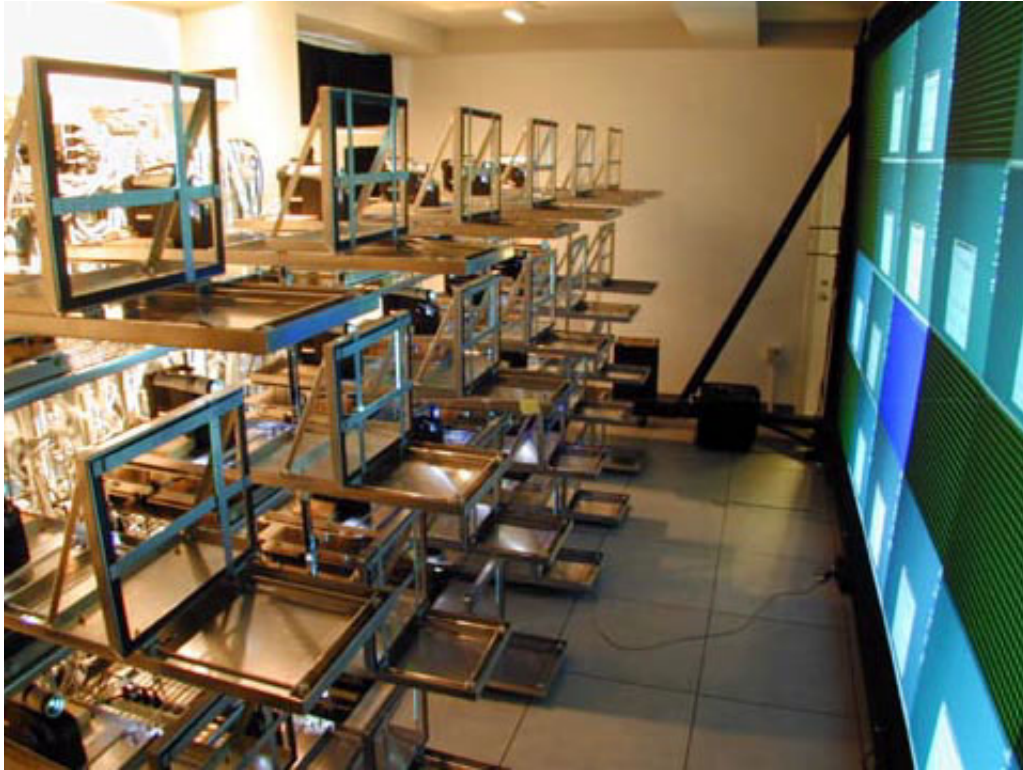
Figure 2.4: A rear view of the Princeton Scalable Display Wall showing 24 portable DLP projectors projecting onto a Jenmar Blackscreen.
