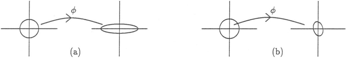
Figure 6: (a) Volume preserving flow. (b) Dissipative flow.
