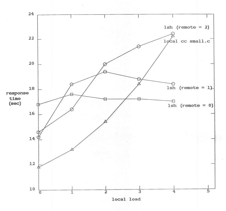
Figure 5. Lsh Performance: compile of small.c, diskless workstations
