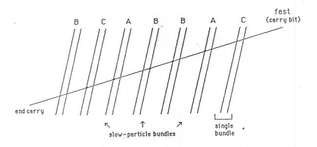
3. An example of the form of a carry-ripple adder. The fast particle travels through the slow-particle bundles, propagating the carry bit.
