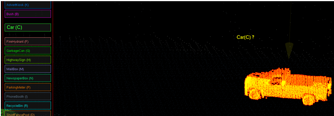
Figure 3.5: Machine-predicted label for a selected unconfirmed object is hovering above the center of the screen and its button is expanded in the label menu.
