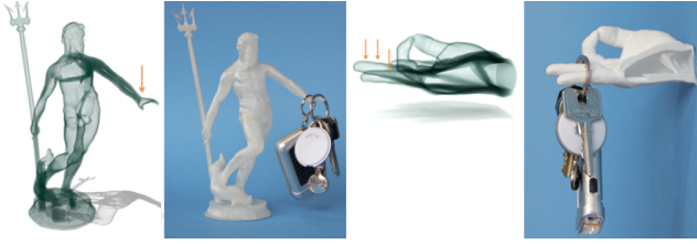
Figure 3: Example results from the method introduced by Wu et al. [WDW15]. Both models were discretized with several million elements, and optimized in a few minutes.
