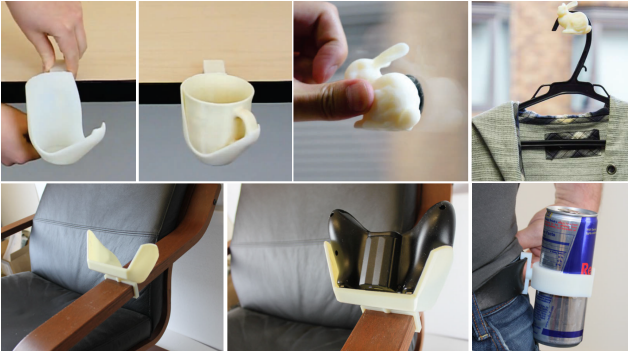
Figure 6: Examples of the automatic generation of various grippers and holders, according to the method proposed by Koyama et al. [KSS*15]. From left to right and top to bottom: a mug holder at desk edges, a bunny-shaped coat hanger connected by suction to a window, a game controller holder on a chair arm, and a two-sided holder, connecting to a belt and a soda can.
