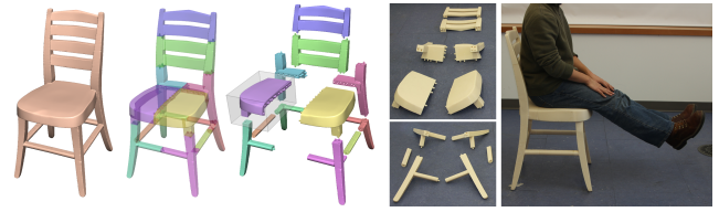
Figure 9: In order to allow for fabrication of objects larger than the printing volume, a partitioning method is proposed to cut and connect the pieces in a structurally sound way [LBRM12].
