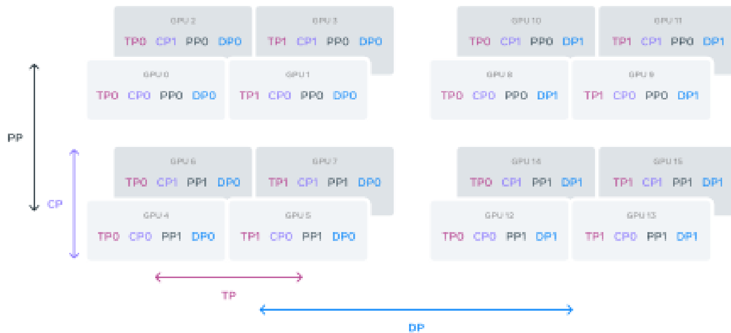
Figure 5 Illustration of 4D parallelism. GPUs are divided into parallelism groups in the order of [TP, CP, PP, DP], where DP stands for FSDP. In this example, 16 GPUs are configured with a group size of |TP|=2 , |CP|=2 , |PP|=2 , and |DP|=2 . A GPU's position in 4D parallelism is represented as a vector, [D_1, D_2, D_3, D_4] , where D_i is the index on the i -th parallelism dimension. In this example, GPU0[TP0, CP0, PP0, DP0] and GPU1[TP1, CP0, PP0, DP0] are in the same TP group, GPU0 and GPU2 are in the same CP group, GPU0 and GPU4 are in the same PP group, and GPU0 and GPU8 are in the same DP group.
