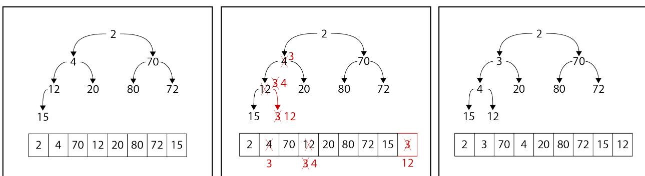
Here are the steps for removing the minimum from the min-heap at the end of the previous example.
