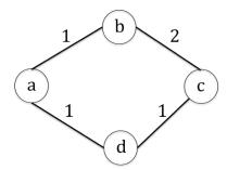
4c) Using the same figure as in question 4b), suppose the network operator is taking link d-c (and c-d) down for *planned maintenance*. The network operator wants to temporarily set the weight of the link to a higher value, to coax nodes to move away from paths that use the link without creating any blackholes or loops. What is the (minimum) sequence of weight settings for the link that ensures no packets destined to node c experience a blackhole or loop? (*3 points*)
