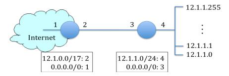
For example, the ISP forwards all packets with destination addresses in 12.1.0.0/17 out link #2 toward the campus edge router. Both routers include a default forwarding entry 0.0.0.0/0 that can match any destination IP address.
