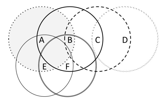
Consider the wireless topology above, comprised of 6 nodes. Circles around each node illustrate their transmission range, e.g. A's range is shown by the dotted, shaded circle. Assume that if the transmissions of two nodes' will interfere at a location if and only if they transmit at the same time and their transmission areas overlap. In these problems, assume that losses only occur due to collisions.
