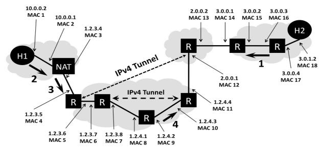
The above figure shows a network topology. The LAN on the left uses a NAT to connect to the Internet and includes a client host H1. The LAN on the right includes a webserver H2. Packets between the two endpoints are routed along the path shown by a heavy dark line, which includes two IPv4 tunnels. All packets that traverse the path use both tunnels. The various network interfaces have IP and MAC addresses as shown.
