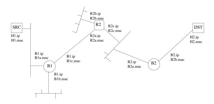
Above is a picture of a network with 2 bridges and 1 router. Each interface is labeled with both an IP address and a MAC address. Imagine that host H1 is sending a packet to host H2. Please answer the following questions about this figure:
